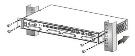
Figure 3-3 NCT480 Mounting Diagram.
